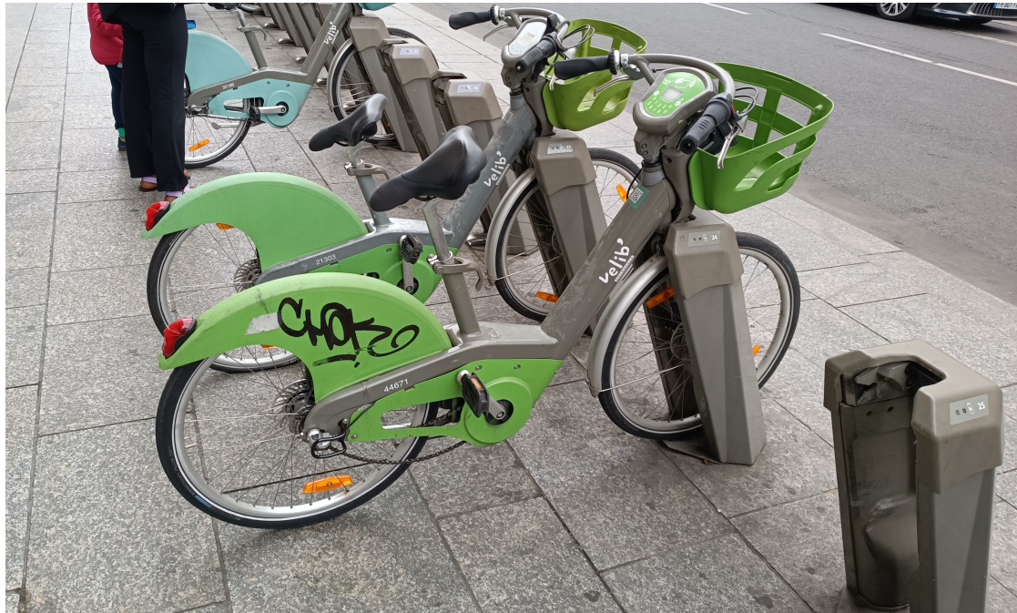
Figure 1: Two Vélib' bicycles, both have their seat turned to indicate they are broken. The chain of the closest one is drooping, which is an additional indicator for those familiar with bicycles.
