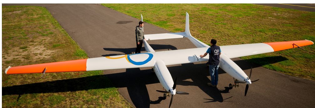
Figure 2. Ampyx Power’s AP3 with a wingspan of 12 m and a wing surface area of 12 m 2 during runway testing at Breda International Airport in May 2021 (photo courtesy of Ampyx Power B.V.).
