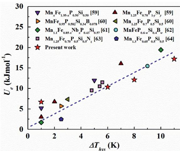
**Fig. 7.** Ashby-like plot demonstrating the relationship between the elastic strain energy  $U_e$  at  $T_c$  and the thermal hysteresis  $\Delta T_{hys}$  for the  $(\text{Mn},\text{Fe})_2(\text{PSi})$  alloys. The dashed line is a guide to the eyes.
