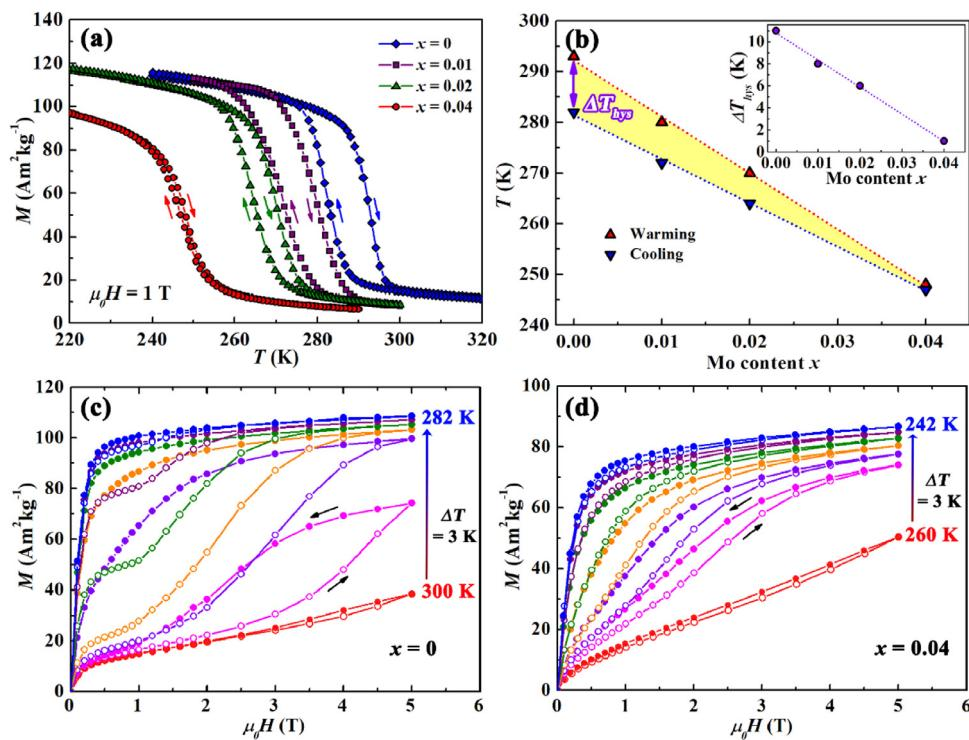
**Fig. 1.** (a) Temperature-dependent magnetization measured in 1 T for the  $\text{Mn}_{1.15}\text{Fe}_{0.80-x}\text{MoxP}_{0.45}\text{Si}_{0.55}$  alloys. (b) Curie temperature as a function of the Mo content derived from the thermomagnetic curves. The dependence of thermal hysteresis on the Mo content is shown in the inset of (b). Isothermal magnetization/demagnetization curves for the  $x = 0$  (c) and  $0.04$  (d) alloys.
