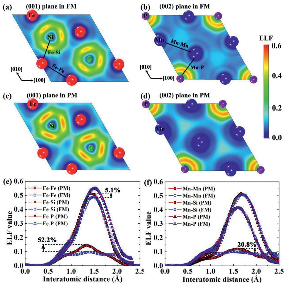
**Fig. 8.** Calculated ELF contour maps on the Fe-Si and Mn-P layers in (a, b) the FM and (c, d) the PM states of the  $(\text{Mn}, \text{Fe})_2(\text{P}, \text{Si})$  alloys. Line profiles of the ELF values (e) between Fe and its nearest neighbors and (f) between Mn and its nearest neighbors. The stoichiometry of  $\text{MnFeP}_{1/3}\text{Si}_{2/3}$  is assumed in the supercell for simplicity of the calculations.
