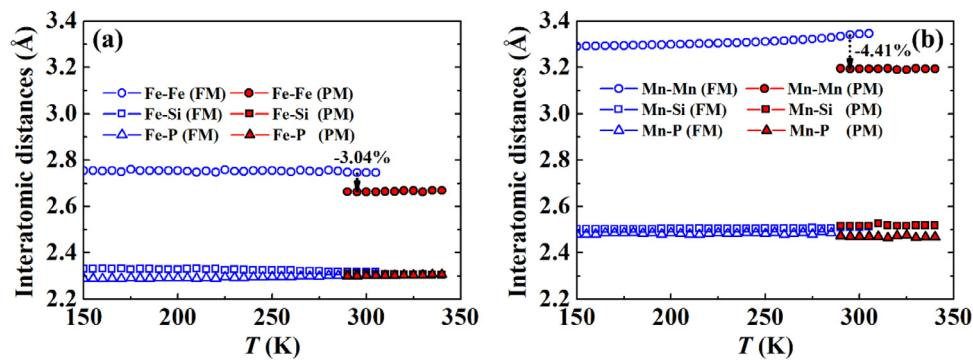
**Fig. 9.** Thermal evolution of interatomic distances extracted from neutron diffraction for the  $\text{Mn}_{1.15}\text{Fe}_{0.80}\text{P}_{0.45}\text{Si}_{0.55}$  alloy. The errors on the refined distances are smaller than the symbol size.
