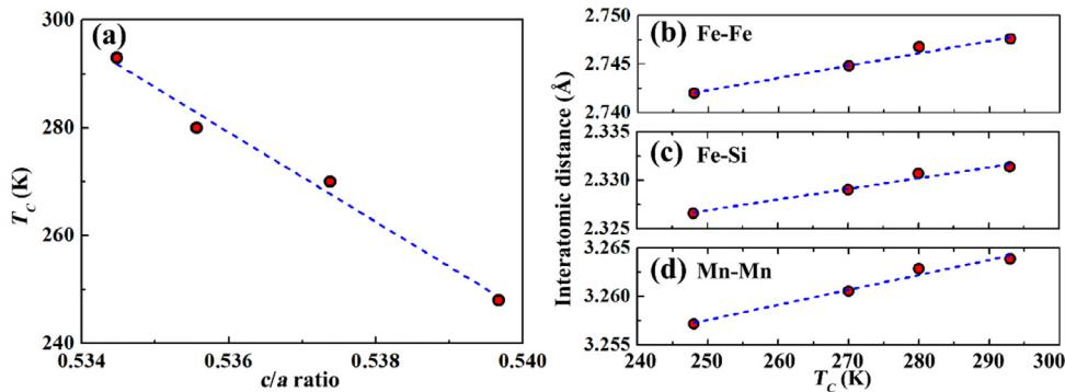
**Fig. 10.** (a) The relationship between the  $T_c$  of the FM-to-PM transition and the  $c/a$  ratio of the hexagonal structure at 200 K for the  $Mn_{1.15}Fe_{0.80-x}Mo_xP_{0.45}Si_{0.55}$  alloys. (b-d) The nearest interatomic distances at 200 K to  $T_c$ . The errors on the  $c/a$  ratio and the interatomic distances are smaller than the symbol size.
