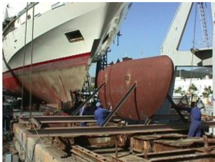
Figure 5. Nesting of a bulb on an existing yacht with conventional bow.
