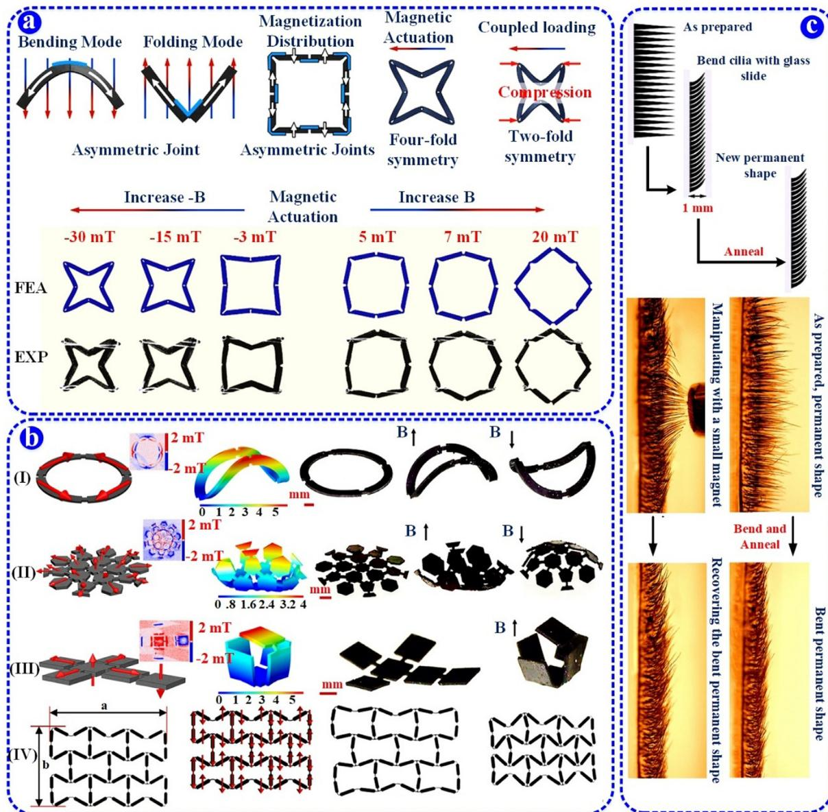
**Fig. 14.** Applications of MRSR in metamaterials. (a) FE simulation and experiment of the deformation mode of the architected structures under the compression loading at different discrete magnetic field [310]. (b) Reprogrammable 3D reconfigurable structures [4]; I) a four-ligament ring, II) a half-sphere, III) a cubic box and IV) an auxetic metamaterial. (c) a reconfigurable cilia [321] a schematic drawing of the programming of the Irogran magnetic cilia.
