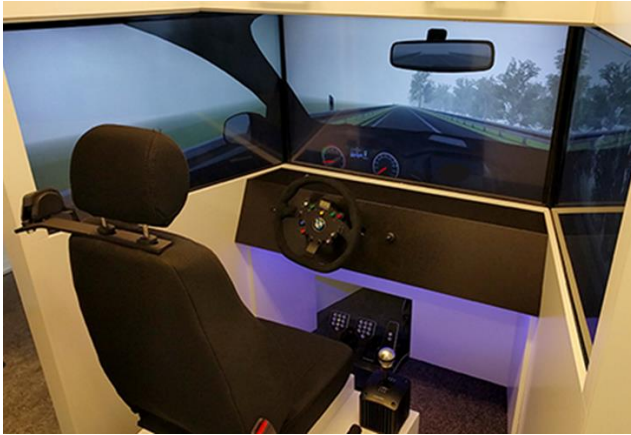
Figure 3-2 The fixed-based driving simulator.
