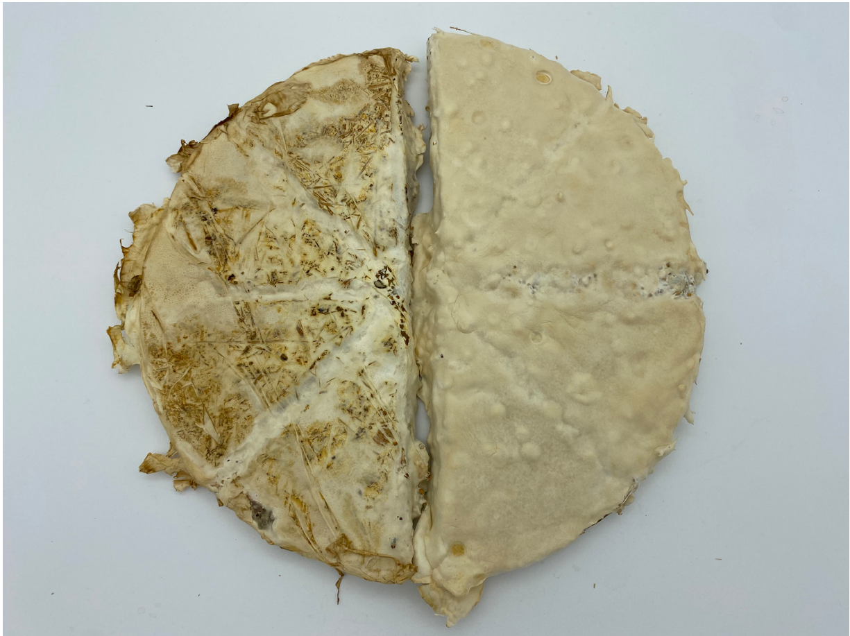
Figure 11. Exploration of spraying extra nutrients thus allowing a layer of fungal skin to grow over. See left verses right, both composites were grown in the same mould. The right had extra nutrients sprayed over
