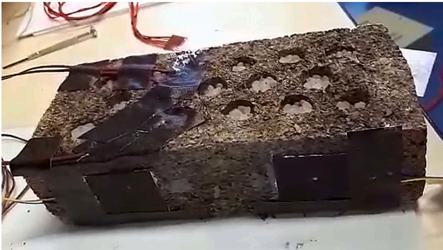
Fig. 6c. View of the brick with holes filled by PCM.
