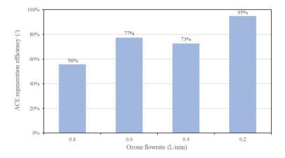
Fig. 6. The influence of gas flow on ACE regeneration efficiency of 900 mg ozone dose
