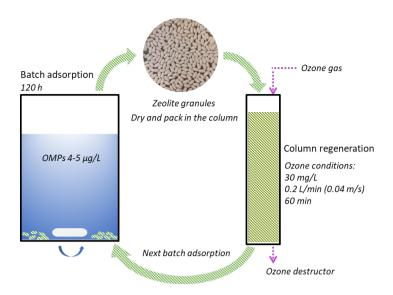
Fig. 1. Sequential adsorption-regeneration procedure
