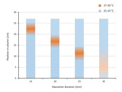
Fig. 6. Heat release zone movement in the column during ozone-based regeneration
