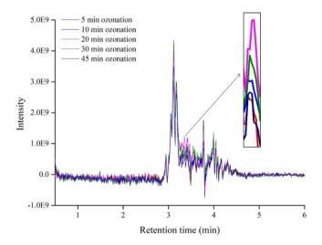
Fig. S2. Total ion choromatogram acquired over a mass range of m/z 50 – 400 in positive ion mode. Liquid samples taken after methanol extraction of granules treated by varying ozonation durations.
