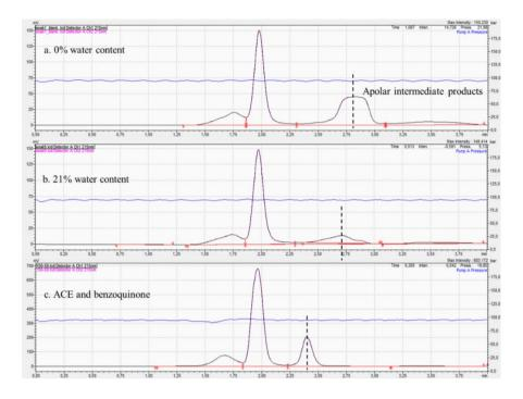
Fig. 5. HPLC peaks: a. extraction from granules with 0% water content; b. extraction from granules with 21% water content; c. samples of ACE and benzoquinone prepared with methanol
