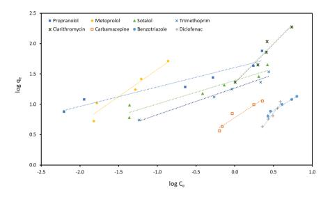
Fig. S2. Adsorption isotherms of the target OMPs on zeolite granules, Freundlich model fitting
