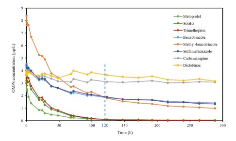
Fig. 2. The concentrations of OMPs as a function of loading time (initial concentration of OMPs at 4-5  $\mu$ g/L, zeolite granules dosage at 0.5 g/L)
