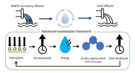
Fig. 3. Advanced wastewater treatment process
