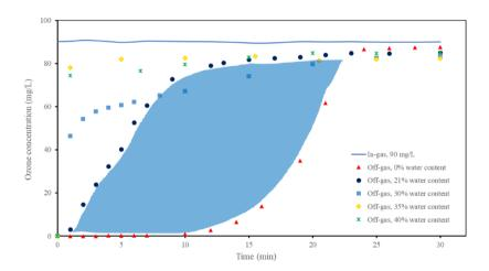
Fig. 4. Ozone concentration of in-gas and off-gas as a function of time under different water content
