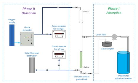
Fig. 2. Two phases setup:
