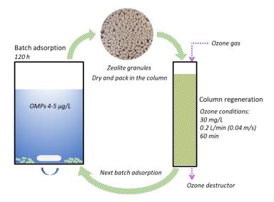
Fig. 2. Sequential adsorption-regeneration procedure
