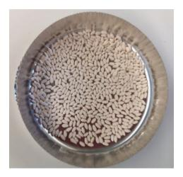
Fig. 1. Printed zeolite granules (after sintering at 950 °C)
