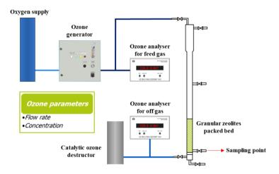
Fig. 1. Experimental setup of big column experiments
