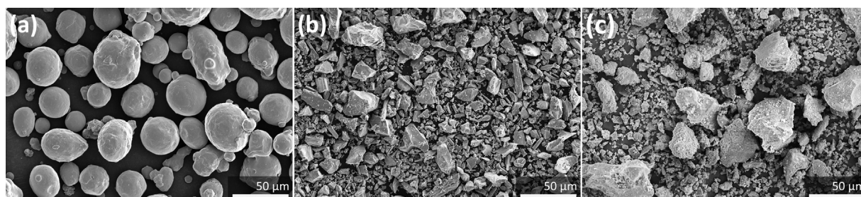
Fig. 1. The morphologies of (a) iron, (b) manganese, and (c) akermanite powders.
