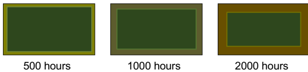
Figure 2. Schematic representation of the oxidized EMC layer at the cross sections of isothermally aged bar-shaped EMC specimens.
