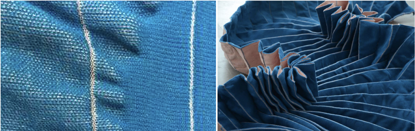
Figure 6: Dynamic Folding Knits by Victoria Salmon [151] is an example of a morhic textile-form that changes in design/production-time. The density of the knit structure is transformed (left) when heat is applied to the thermoplastic yarn used. This stiffens the structure and enables the embedded folds (right) to activate. Image credit: Victoria Salmon.
