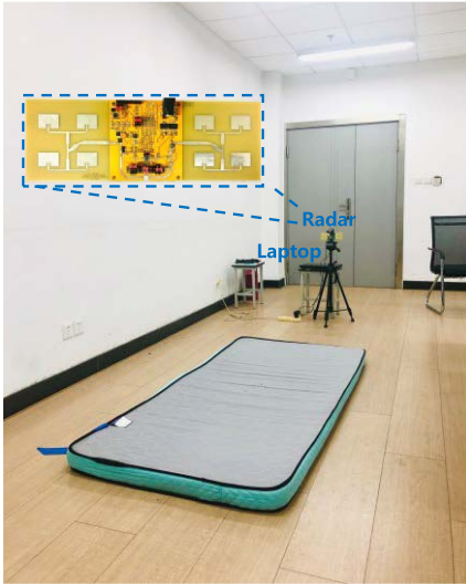
Fig. 6. Experimental setup with radar system and area where the activities are performed, including a mattress for controlled falls.
