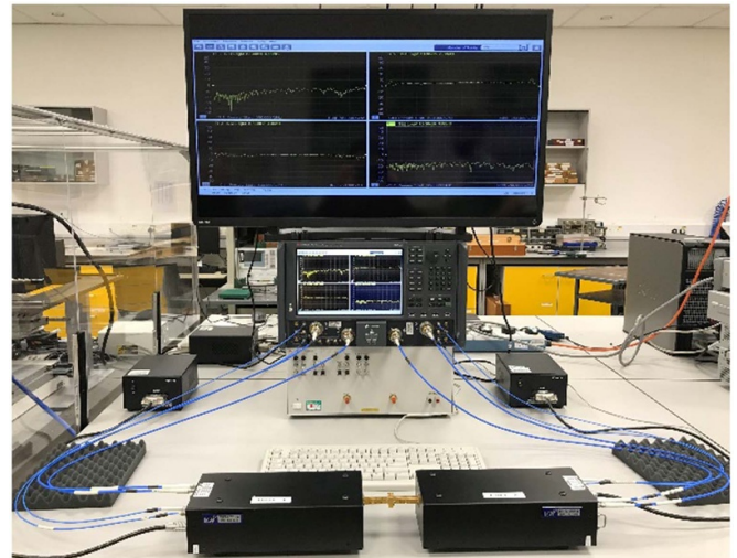
Figure 28. An example THz waveguide-based system comprising a dual source vector network analyser (VNA), along with two frequency extender heads shown in the foreground.
