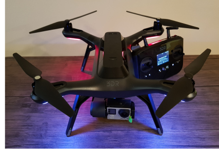
Fig. 12. 3DR solo drone that was used as part of the final test set.
