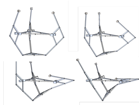
Fig. 8. CAD model of the current manipulator transitioning from translation mode to mixed freedom mode. As the center moves away from the center's vertical axis the tilt angle increases.
