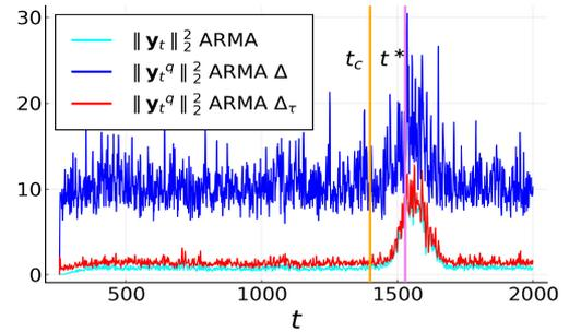
Fig. 3. Squared norm of unquantized and quantized filtered streaming graph signals for the change point detection problem, when using the ARMA<sub>4</sub> filter of NOUGAT algorithm [53], where  $N = 200$ ,  $a_s = 300$  m,  $\mathbf{S} = \mathbf{L}_n - \mathbf{I}$ ,  $\Delta_0 = 1.19$ ,  $\chi = 5$  bits. The change-point is set at  $t_c = 1400$  and the NOUGAT detection is expected at  $t^* = t_c + 128$  for the same NOUGAT parameter values of [53].
