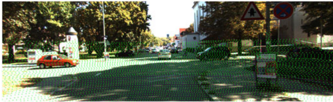
Fig. 5. LiDAR scan (green) projected into reference RGB image. The vertical field of view of the KITTI LiDAR sensor only covers a range up to a few degrees over the horizon. Nevertheless, the resulting scene completion training targets cover objects at more than 2m over the ground since they are accumulated from more distant ego-positions.
