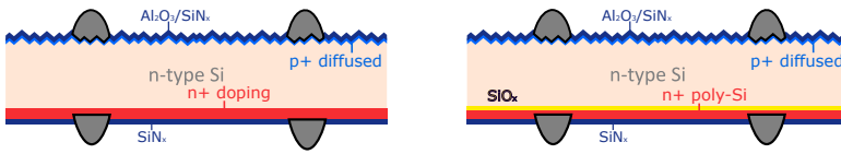
Figure 2.6: Schematic structures of an n-PERT (left) and an i-TOPCon solar cell (right).
