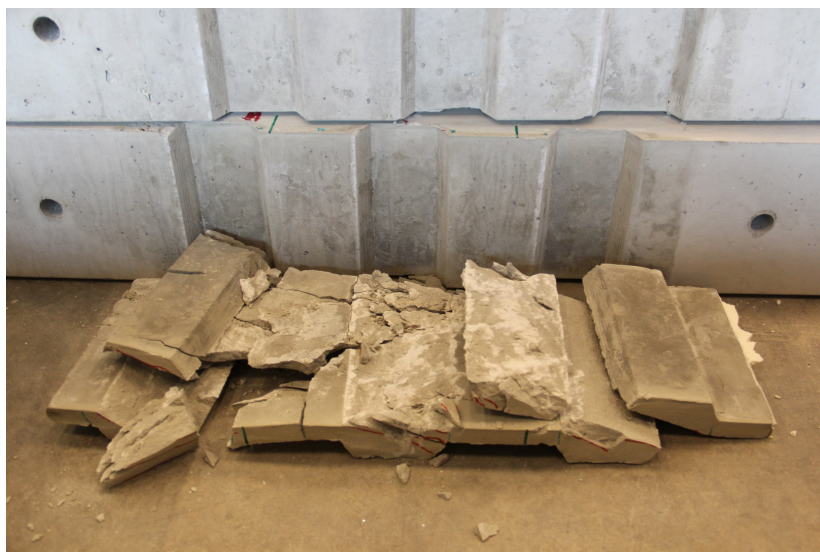
Figure E.3: Specimen 1-3: Dismantled specimen (Tiksomortar k70)
