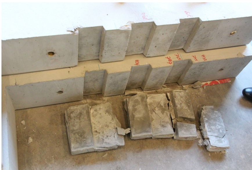
Figure E.5: Specimen 2-7: Dismantled specimen (Tiksomortar K70)
