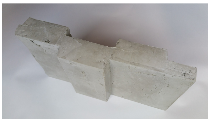
Figure 4.3: The mortar filling after demoulding
