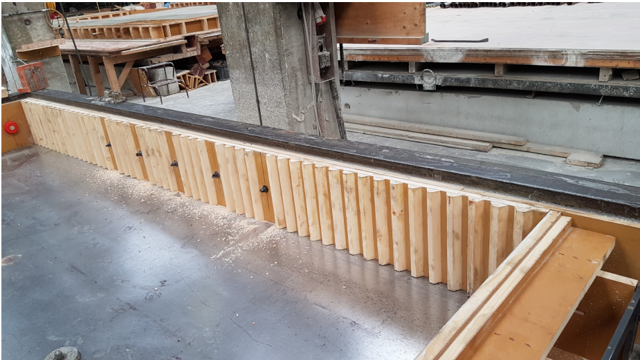
Figure 3.5: Wooden ribbings in the edge side formwork for the Aligned small shear key connection of a precast concrete large panel element
