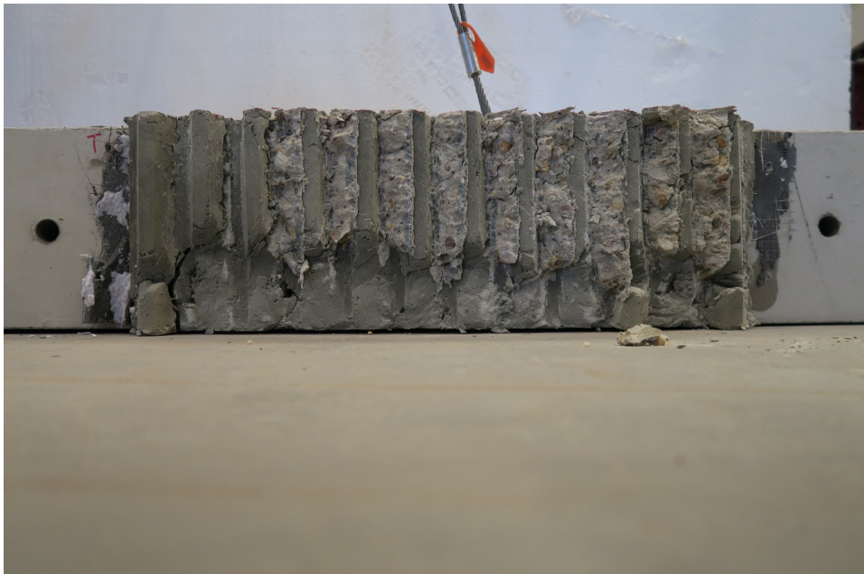
Figure E.11: Dismantled specimen: Specimen 3-5 (top) and 3-6 (bottom)
