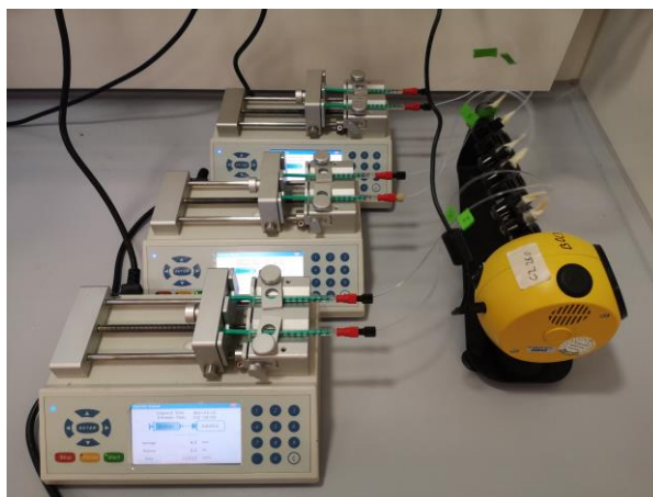
Figure S3.1. Reaction set-up for the enzymatic epoxidation of cis - \beta -methylstyrene. On the left, syringe pumps for continuous t BuOOH supply. Syringes are connected to tubes which lead to the reaction mixture inside GC vials on the right.
