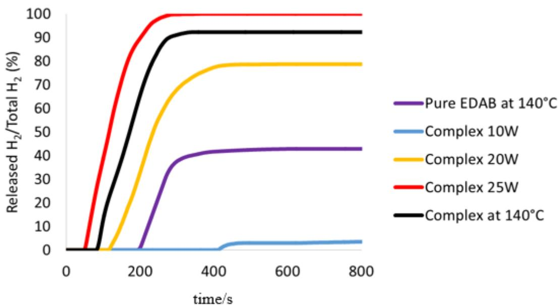
**Figure 6.** H<sub>2</sub> flow during the liberation tests
