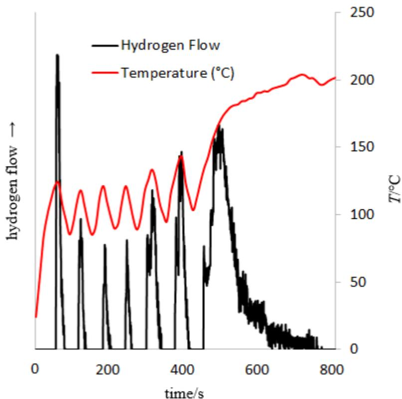
**Figure 7.** H<sub>2</sub> flow and sample temperature during a liberation test with microwave pulses of 25W
