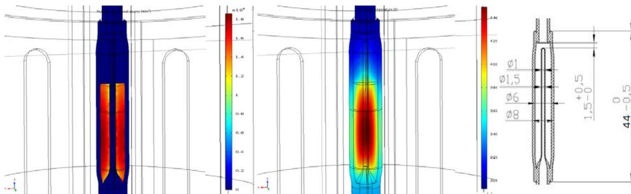
**Figure 4.** Simulation results. On the left, heat source ( $\text{W/m}^3$ ); on the centre,  $T$  (K); on the right, dimensions of the glass vessel
