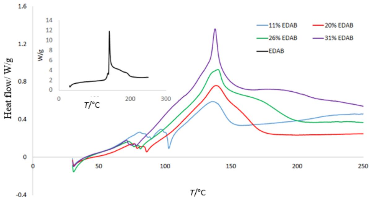
**Figure 3.** DSC profile of EDAB and the impregnated complex before and after H<sub>2</sub> release.
