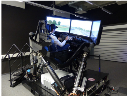
Figure 1: BMW's small hexapod simulator "Orange Vector".
