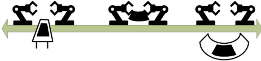
Figure 1.1: Grip, transfer and drop phases of the pick-and-place process. Adapted with permission from: Schuster *et al.* [5].
