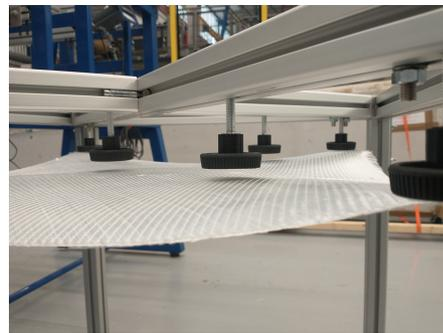
Figure 5.2: Frame with a 550 x 550 mm reinforcement suspended from the pick-up points
