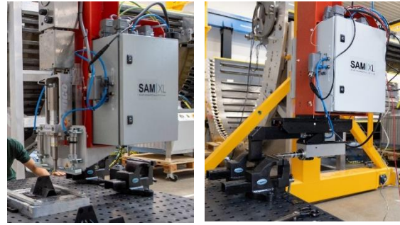
Fig. 4: Ultrasonic welding EEF in the CTS configuration (left) and CTF configuration (right) on a static test bench.
