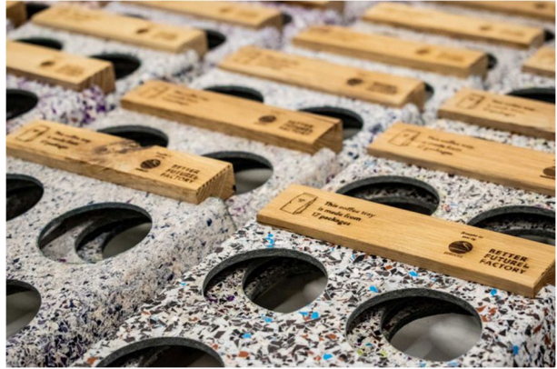
Fig. 2 Coffee trays made from recycled coffee packages by Better Future Factory. https://betterfuturefactory.com/portfolio_page/selecta-coffee-trays/
