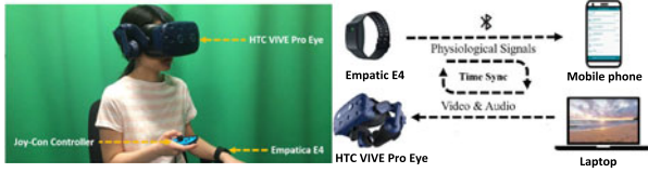
Fig. 5. The experimental setup and annotation interface for CEAP-360VR [82].
