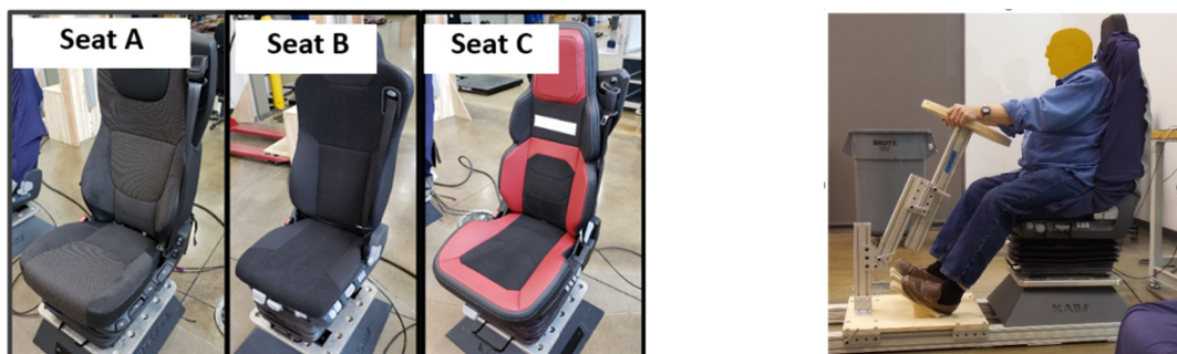
Figure 1. Left side - the three seats tested in the study. Right side - a subject sitting in the simulated truck cab.
