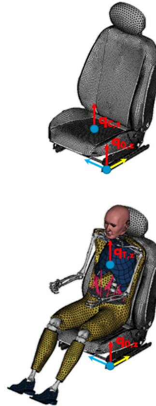
Figure 3: Comparison of Seat Transmissibility at Cushion Surface (top) and at Torso (bottom)
