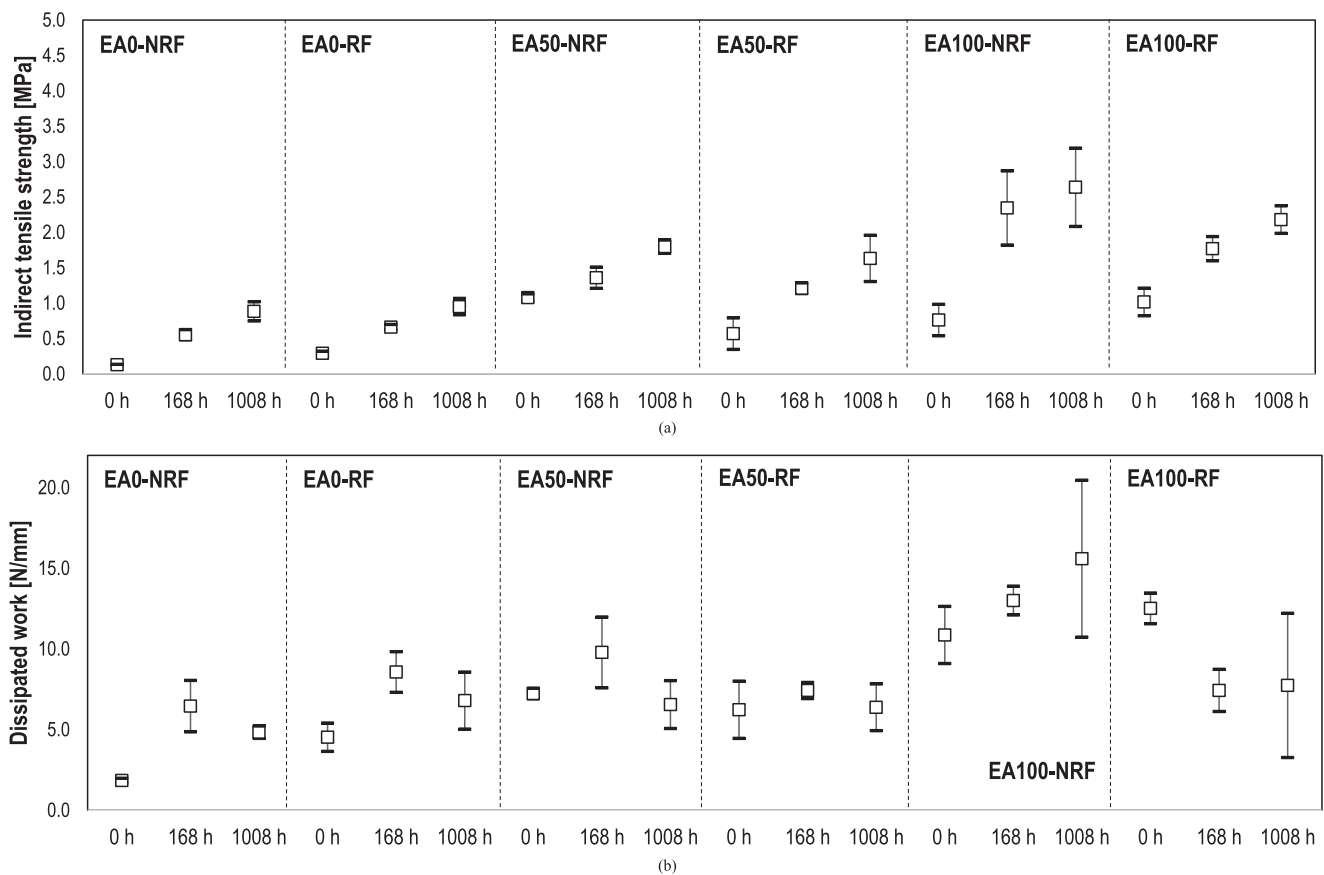
Figure 8. Change of (a) tensile strength and (b) dissipated work of long-term aged materials due to water conditioning.
