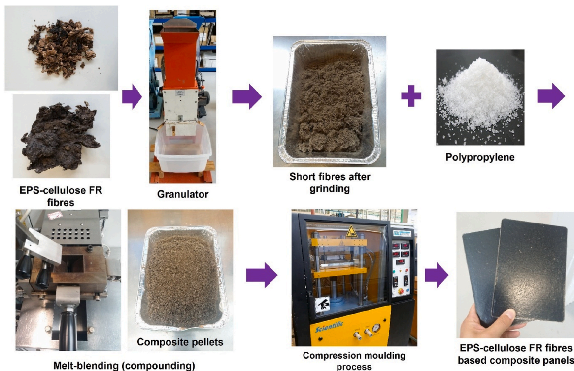
Fig. 1. Manufacturing process of EPS-cellulose FR fibres/PP composites.
