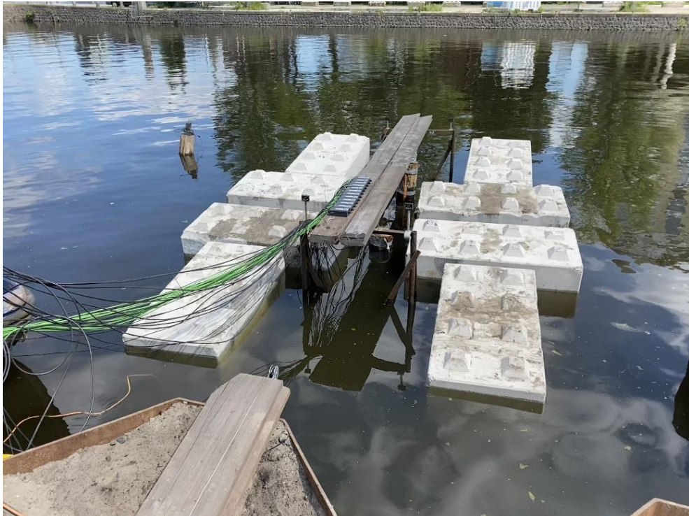
Figure C.3, Photograph of lateral pile group experiment with top load. LEGIO-blocks are visible above the water level.
