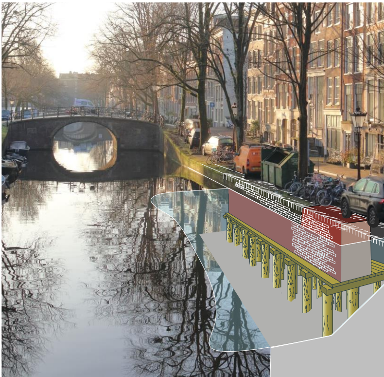
Figure 1.4, Cutaway drawing of historical quay wall structure. Photograph taken at Reguliersgracht, Amsterdam (Mart-Jan Hemel, 23 December 2021).
