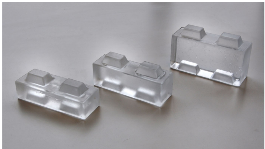
Fig. 30 Interlocking, dry-assembly glass bricks developed by Oikonomopoulou, Bristogianni and Barou for the 3TU.bouw Lighthouse project: Restorative Glass
