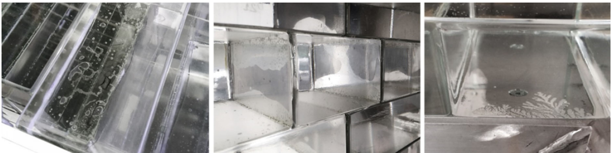
Fig. 18 Common flaws occurring in the adhesive layer: air gaps, capillary action and dendroid patterns
