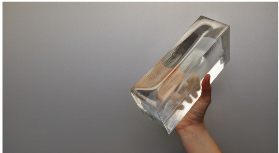
Fig. 11 Glass bricks rapidly cooled (prior to annealing) in vertical orientation. The natural shrinkage is evident besides the top surface , also along the larger surfaces
