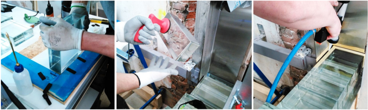
Fig. 26 From left to right : Bonding of the steel plate to the corner brick. Positioning of the brick by a suction cup holder. Application of the semi-elastic polymer
