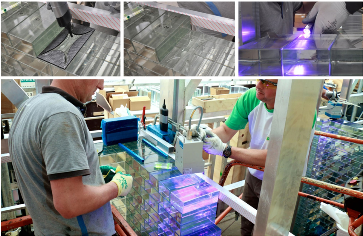
Fig. 19 Bonding steps from left to the right : 1. Application of the adhesive with the aid of the PURE® form. 2. Resulting \times pattern. 3. Local hardening of the adhesive by a UV beam light for
