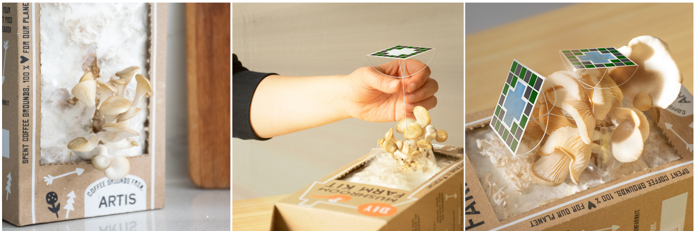
Figure 16: Mushroom Shade : Under excessive sunlight, the EC unit of the interface would darken its colour, casting a protective shadow onto the fungi body underneath. Users can provide care to the mushrooms in a delicate way, by “planting” the Mushroom Shade above each cluster of fruiting bodies.
