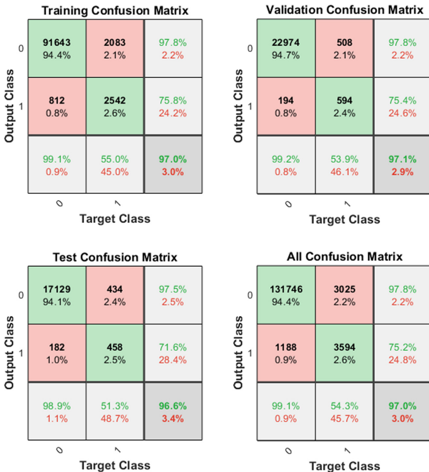
Figure 10.13 Confusion matrix of PRNN for the first architecture with 10 neurons on thermograms.
