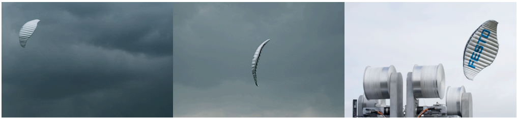
Figure A.1 | Early generation quad-tether ram-air kites developed in collaboration with FESTO (circa 2010) [181].
