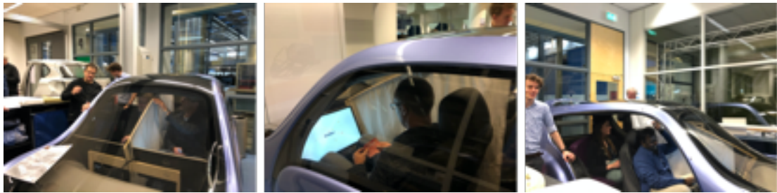
Figure 9 Photographs of the experimental set-up. Left photo: the CMMN car with driver and automation screens and a curtain in between. In the middle photo a driver is looking at the start screen of the experiment. The Right photo shows a participant (ic., Automation) handing a decision card to the Mediator.
