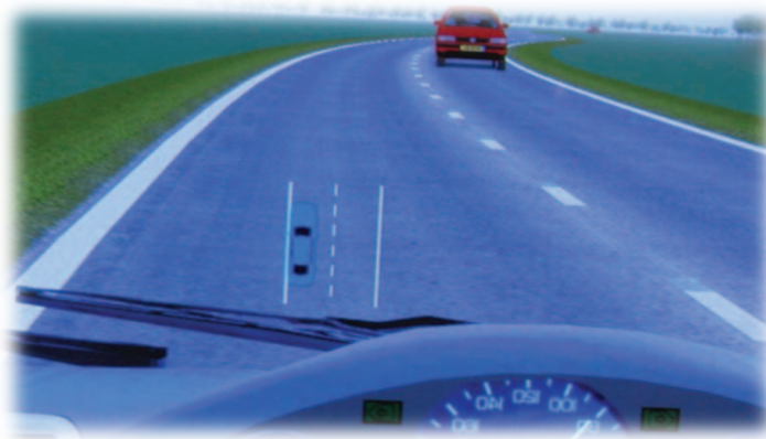
Figure 64 Lane position information projected on the windshield (Dijksterhuis et al., 2012)
