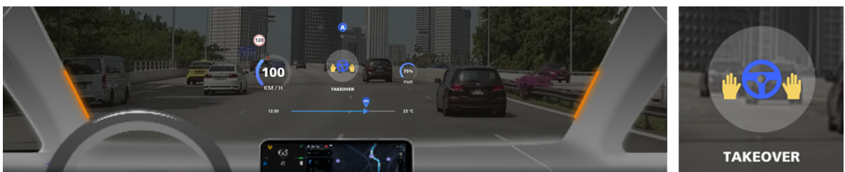
Figure 26 The HUD & light-strip signals during takeover request
