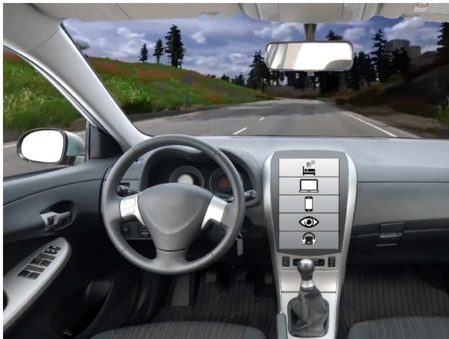
Figure 2: Five icons were designed to communicate the desired driver task. The intended meaning of these icons from top to bottom was: It's allowed to sleep, it's allowed to use your laptop, it's allowed to use your phone, you are required to pay attention to the road, you are required to take control of the steering wheel. Only one icon was presented to a participant at a time.
