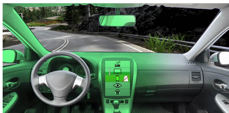
Figure 57 The full HMI concept for the concept group 'show desired driver task', showing a continuous transition from high automation fitness (top panel) to low automation fitness (bottom panel).
