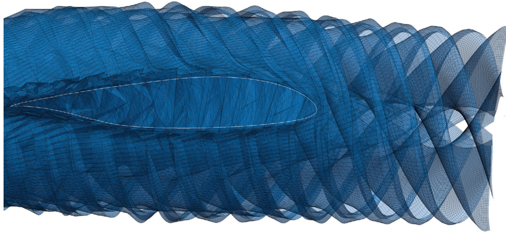
(a) Free wake results. Wake filaments penetrating through wing.
