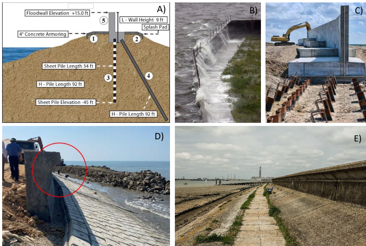
Figure 11: A) A sketch of an L-wall with an H-pile for enhanced stability and a splash pad against erosion. B) a flood wall with the erosion-resistant splash pad in action (USACE, 2019). C) A concrete floodwall during construction in New Orleans, with a foundation of steel sheetpile and H piles (Jonkman et al., 2021). D) A curved or straight nose (parapet) can be used at the top of a floodwall to reflect waves back and reduce overtopping, like here at the Hoang Hoa sea embankment under construction in Vietnam (within red circle) or E) at this seawall in the UK (by Scott Wylie , CC BY licence).
