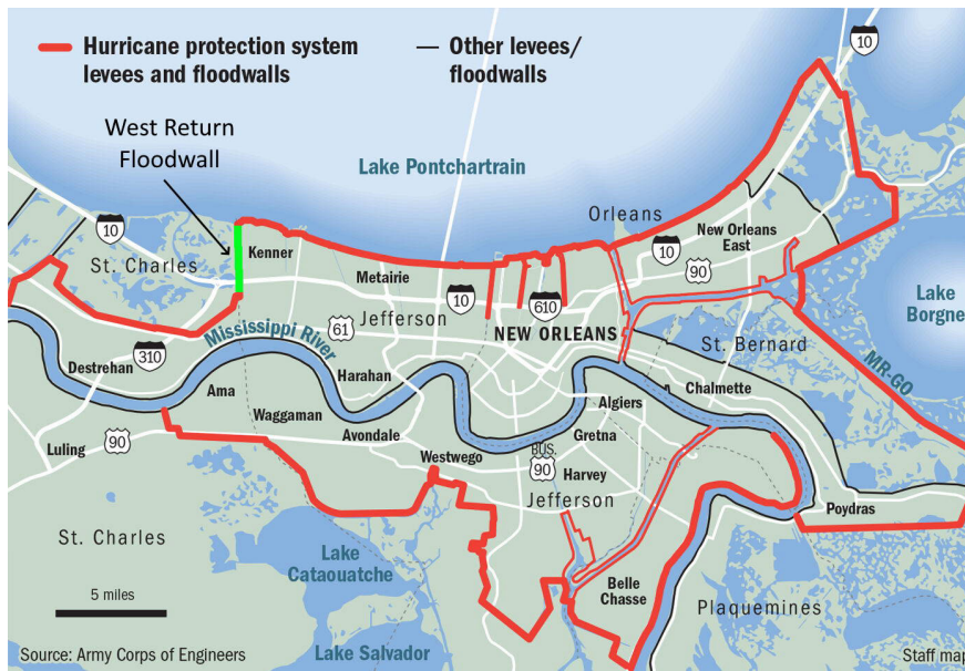
Figure 31: The HSDRRS flood protection system of New Orleans, with the West Return Floodwall indicated in green (adapted from Swenson, 2022)
