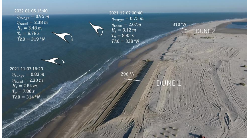
Fig. 1 Aerial photograph of the field site including offshore hydrodynamic conditions during the three campaign storms. The water levels were measured at the Hoek van Holland and Scheveningen stations. The wave conditions were measured at the offshore EuroPlatform station
