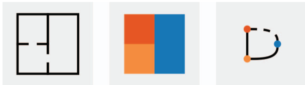
Figure 1. Floor plan representations. Left: Pictorial image. Center: Semantic image. Right: Access graph.
