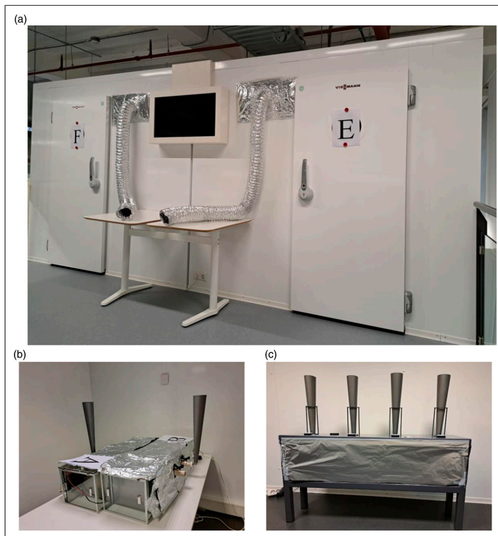
Figure 1. Test environments: (a) test chambers; (b) CLIMPAQs; (c) sniffing table.
