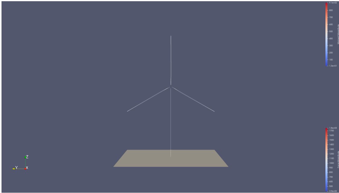
(a) Line representation of the turbine in OpenFAST
