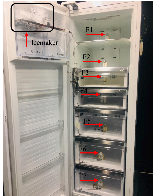
Fig. 4. The location of thermocouples installed inside the freezer.
