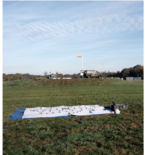
Figure 2: Acoustic array used during the measurement campaign
