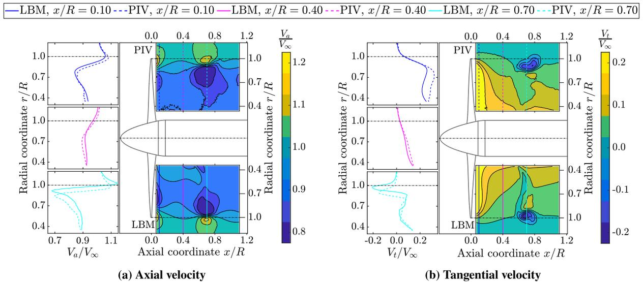
Fig. 9. Comparison of the phase-locked slipstream from PIV data and LBM simulations for the negative thrust condition at  $\phi = 0^\circ$  ( $J = 1.10$ , fine grid).
