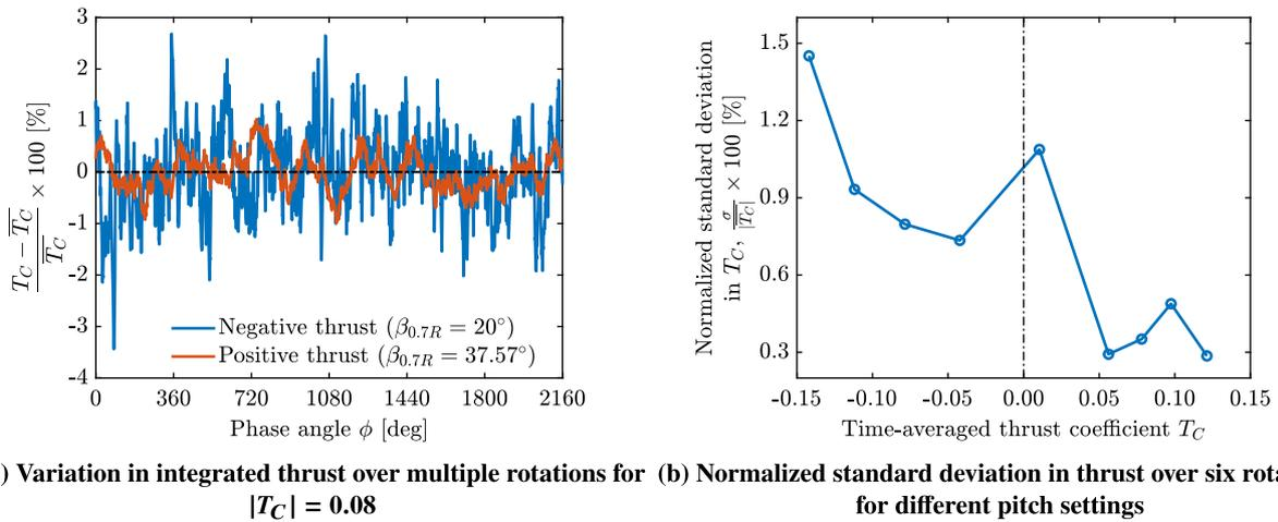
Fig. 17. Time-accurate integrated thrust performance at  $J = 1.34$ .
