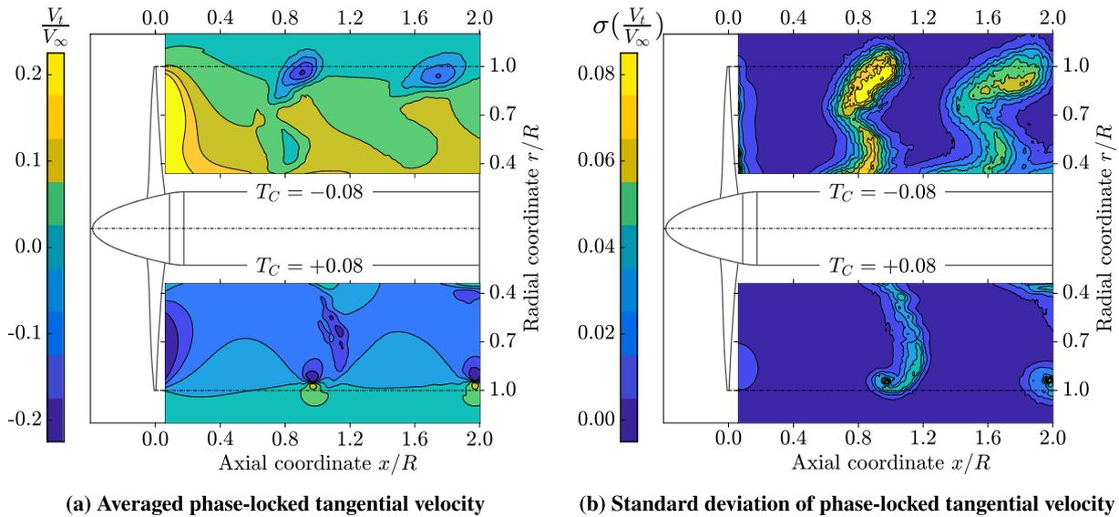
Fig. 19. Comparison of tangential velocity contours in negative ( $\beta_{0.7R} = 20^\circ$ ) and positive ( $\beta_{0.7R} = 37.57^\circ$ ) thrust condition at absolute thrust level of  $|T_C| = 0.08$  (Phase-locked).
