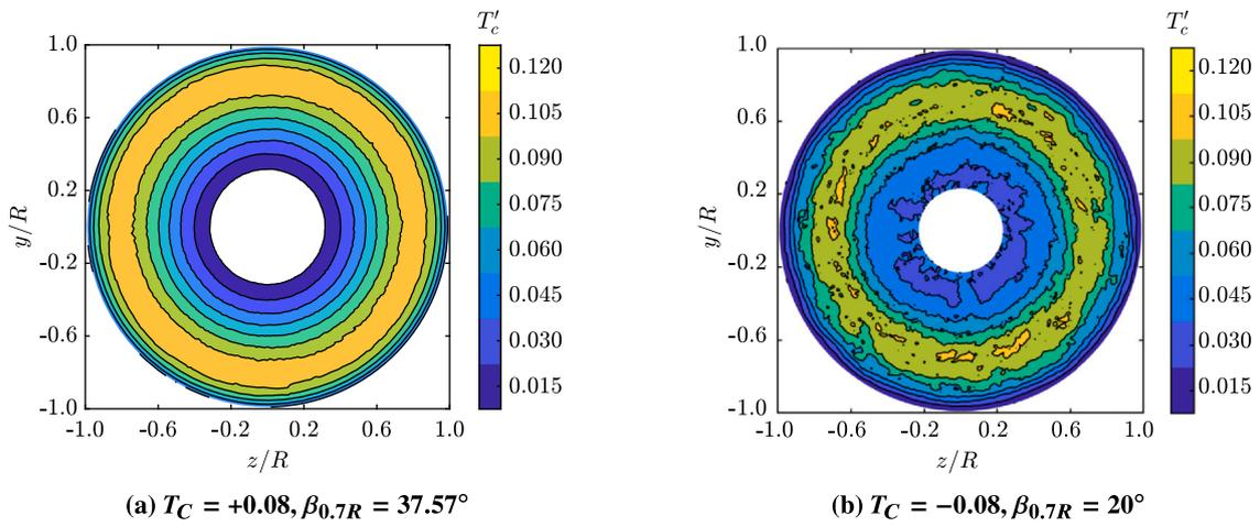
Fig. 16. Radial distribution of instantaneous thrust coefficient ( $T'_c$ ) along the propeller blade span over a rotation as a function of circumferential position for  $T_C = \pm 0.08$  at  $J = 1.34$ .
