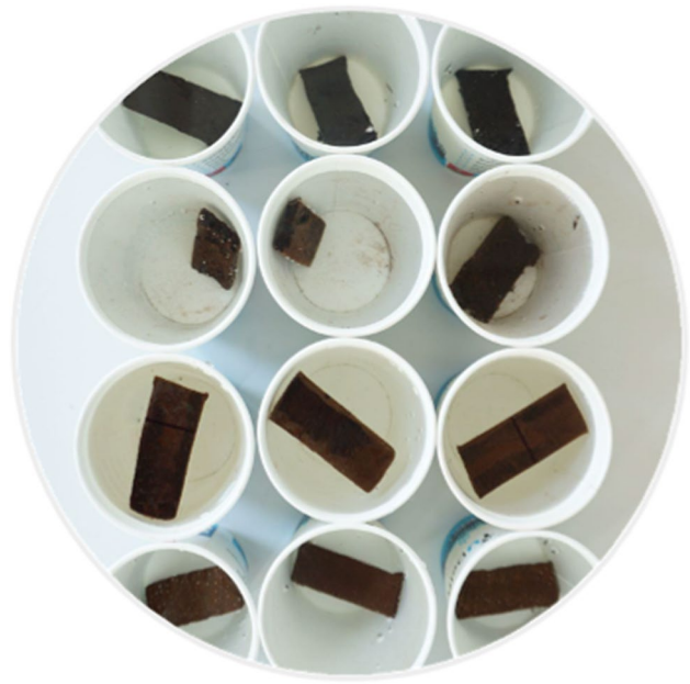
Fig. 5 Water absorption & retaining test (picture by authors)
