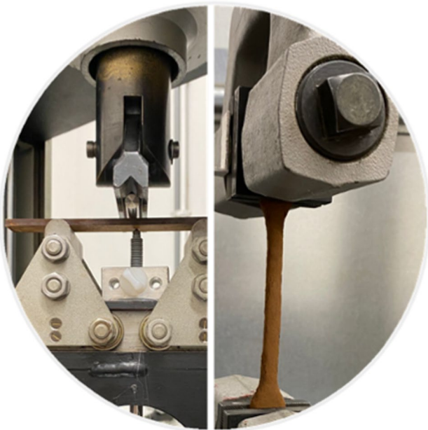
Fig. 4 Tensile & 3 point bending test (picture by authors)
