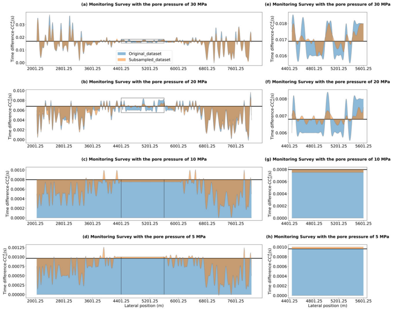
Figure 6. The retrieved time differences in the reservoir using ghost reflections for the monitoring surveys with pore pressure of (a) 30 MPa, (b) 20 MPa, (c) 10 MPa and (d) 5 MPa for all virtual receivers. (e), (f), (g) and (h) Zoomed in results from inside the black rectangles in (a), (b), (c) and (d), respectively. The blue highlighted area shows the time difference using the original data set, and the orange one shows the time difference using the subsampled data set. The horizontal black lines show the calculated time differences.
