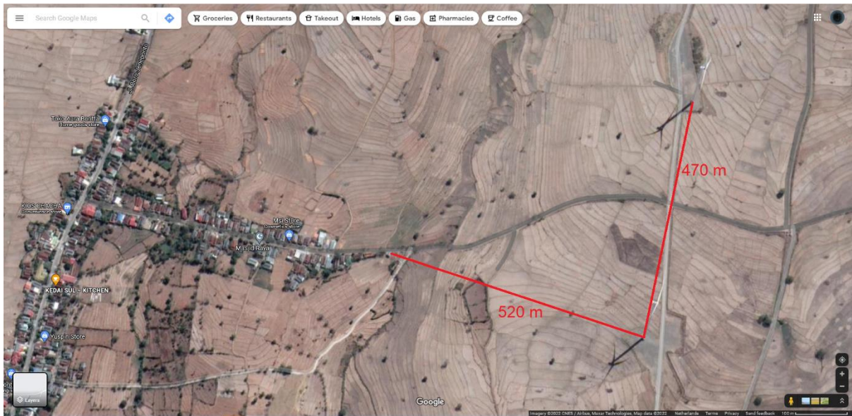
Screenshot of a part of the Jeneponto wind farm in Indonesia from google maps. The distances between turbines and to the closest house were measured with the distance measurement tool of google maps [221].
