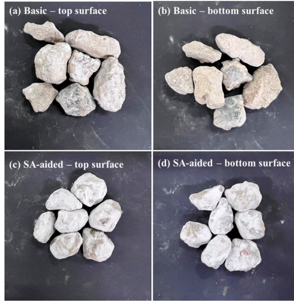
Fig. 9. The (a) top surface of RCA after basic MICP treatment, (b) bottom surface of RCA after basic MICP treatment, (c) top surface of RCA after SA-aided MICP treatment, and (d) bottom surface of RCA after SA-aided MICP treatment.
