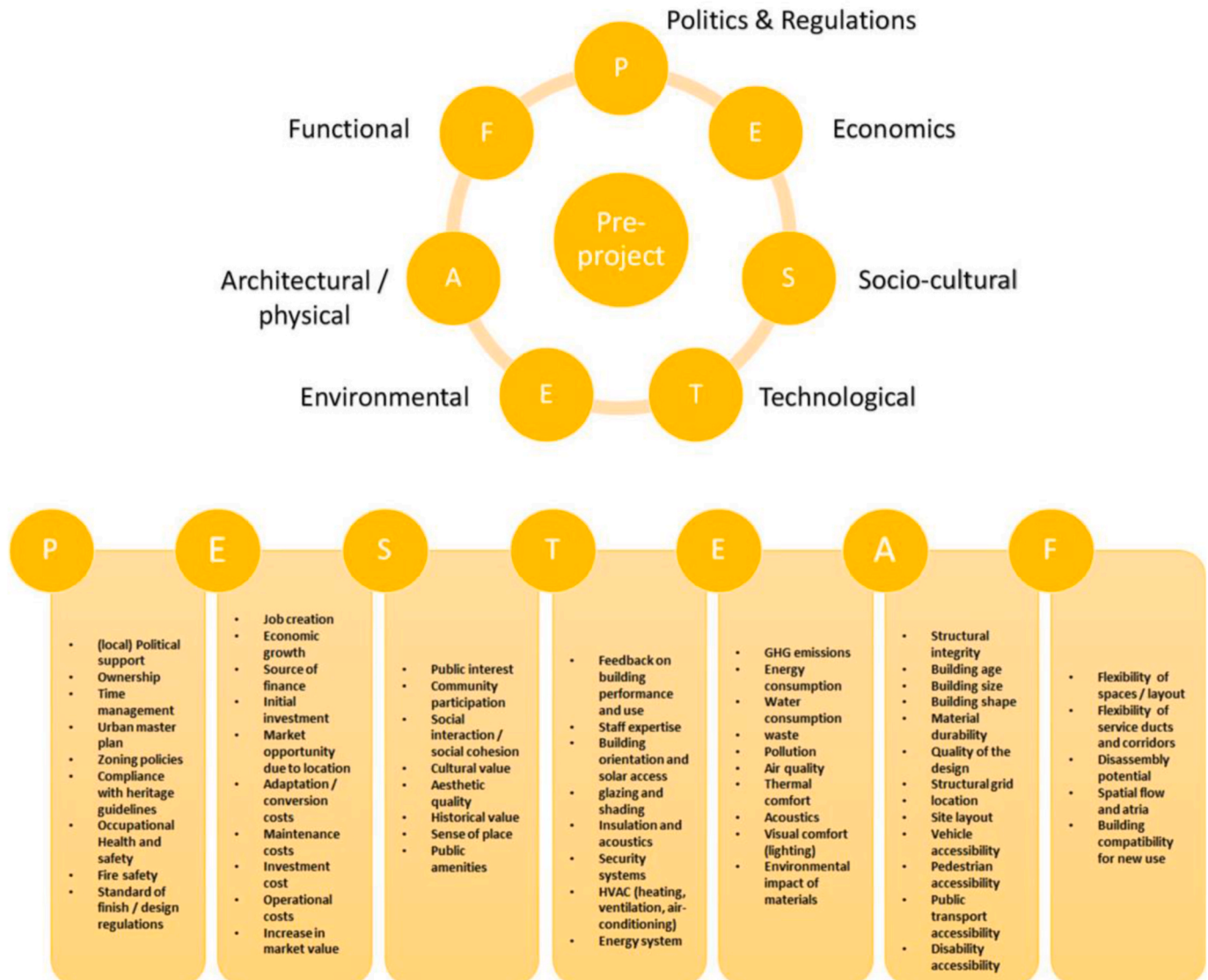
Fig. 2. The decision criteria for adaptive reuse in the pre-project phase.
